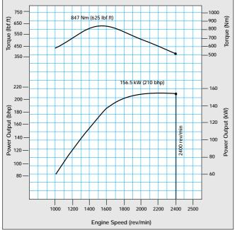
Lower power ratings may not be read from this curve. Other ratings are available contact Perkins Engines Company Limited
