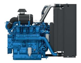
Bore & Stroke (mm) Displacement (L) N° of Cylinders Cylinders Arrangement Fuel System Governor (Gov.) Aspiration (Asp.) 150 x 185 26.1 8 At Vee High Pressure Common Rail / Mechanical ECU / Electronic Turbocharged & air-to-air cooled
